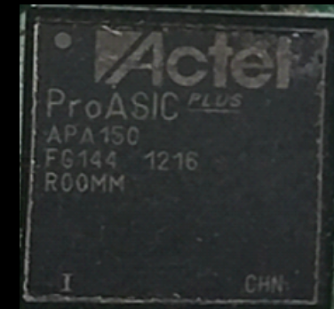
Xilinx Spartan-II FPGA and Actel ProASIC Plus FPGA – programmable logic devices enabling application-specific digital functions.
